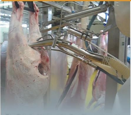
The Robotic Hindquarter Sani Vac replaces the actions of manual steam vacuum sanitisation operations for lamb sheep and goat processing.
