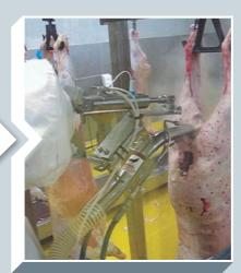
Generally the Vac San operation consists of 4-6 passes, designed to maximise effective use of processing time available and customised to meet plant processing requirements with a range of line positions and design configurations available.
