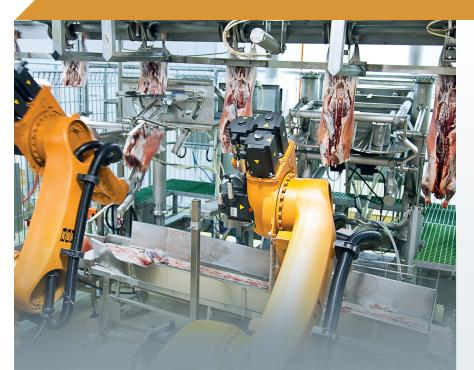
The X-Ray Primal System automates the cutting of lamb primals. The system delivers highly accurate, clean primal cuts superior to anything produced by a human operator.
