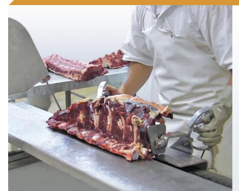
The Striploin Saw delivers the the safest and most efficient means of removing the striploin from the chine bone.
