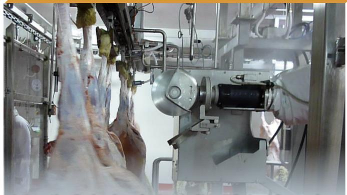
Innovative Technology for Lamb, Sheep & Goat Processing. The robotic brisket cutter replaces current manual brisket shear operations for lamb sheep and goat processing.
